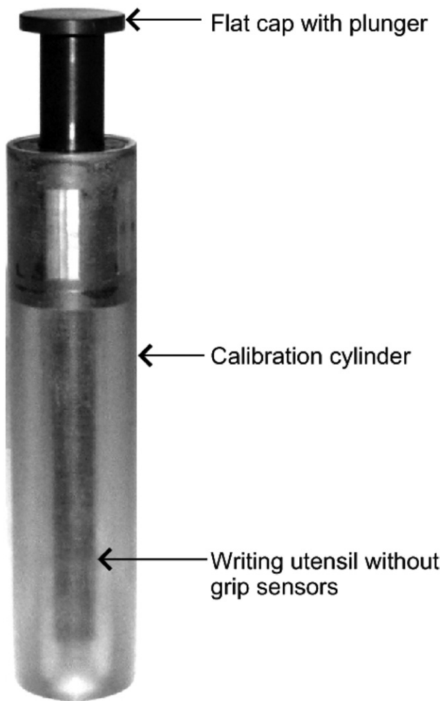
Fig 4. Plunger and cylinder for calibrating normal force measurements. The writing utensil has been inserted into the hollow cylinder. Small weights can be placed on the flat cap to calibrate normal force readings as described in the text.
