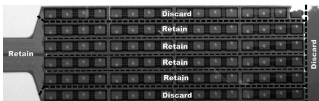
Fig 2. Trimming the model 9811 force sensors for use as grip sensors.
